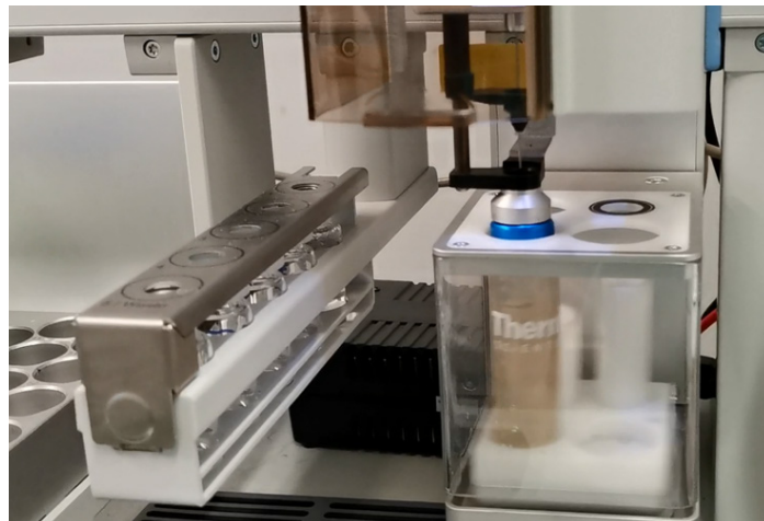
Figure 2. Vortex Mixing tool for automated in-vial liquid-liquid extraction (LLE)
