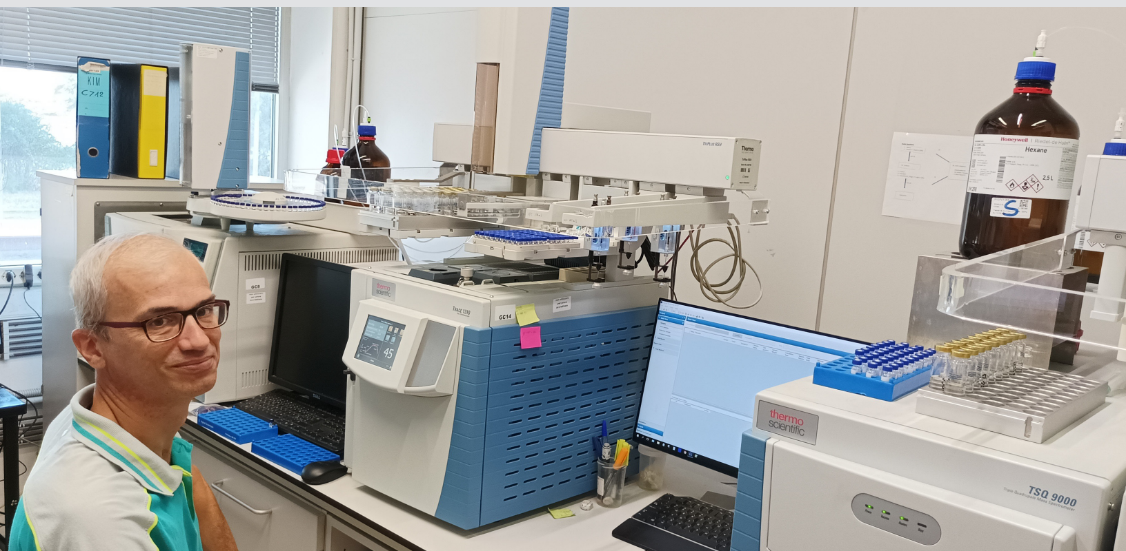
Analytical systems used by VERITAS Integrated Water Service Laboratory for semi-volatile organic compounds (GC-MS/MS) and mineral oil (GC-FID) in water samples with automated liquid-liquid extraction (LLE): Thermo Scientific™ TRACE™ 1300 Series Gas Chromatograph with Thermo Scientific™ iConnect™ Programmable Temperature Vaporizing (PTV) Injector Module for large-volume injection, Thermo Scientific™ TSQ 9000 triple quadrupole GC-MS/MS, with the Thermo Scientific™ TriPlus™ Robotic Sample Handling (RSH) autosampler.
